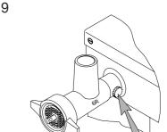
When the meat mincer has been assembled, it is mounted in the attachment engagement hub of the mixer. The meat mincer must be pressed into the attachment engagement hub before the thumb screw is tightened.
