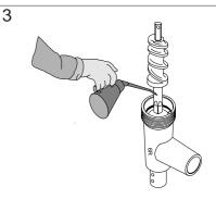
The shaft of the feed screw should be lubricated with grease before the feed screw is inserted into the housing. Use e.g. paraffin oil or castor oil, never salad oil.
