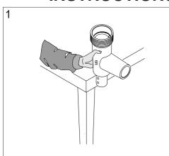
Place the housing on the edge of a table, the opening upwards, when the meat mincer is to be assembled.
