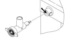
If the feed screw is stuck, when the meat mincer is to be disassembled, it can be pulled out by inserting a hook or a similar tool in the hole of the feed screw shaft.
