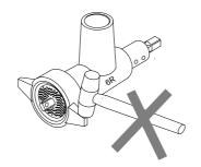
The ring should only be screwed slightly on by hand.
