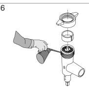
The thread of the housing should be lubricated with grease before the distance ring and the ring are mounted. Use e.g. paraffin oil or castor oil, never salad oil.
