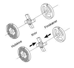
The knife must be replaced or grinded when the wearing surface on the side of the knife is more than **1 mm**. If this is not done, the mixer can be damaged, as
